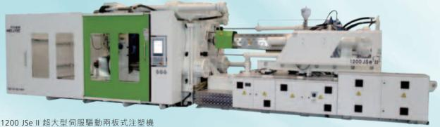
1200 JSe II Ultra Large-sized Servo-driven Two-platen Injection Moulding Machine
