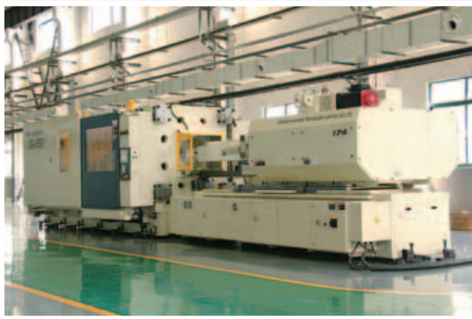
UGe850 All-Electric Injection Moulding Machine
