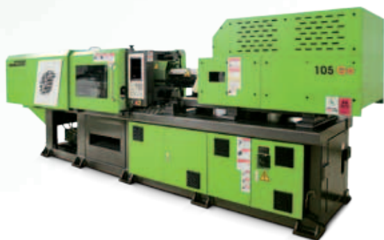
105Gell All Electric Injection Moulding Machine
