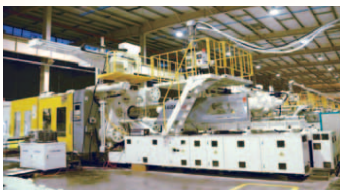
● DONGHUA 1600JSe Servo-Driven Energy Saving Two-Platen Plastic Injection Moulding Machine
