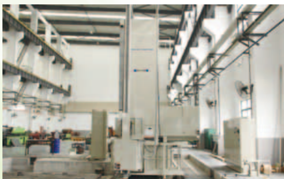
Toshiba BSF-150B CNC Milling and Boring Machine in Wuxi new production base
