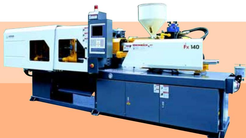
*High Speed, High Precision Series Injection Moulding Machine*
